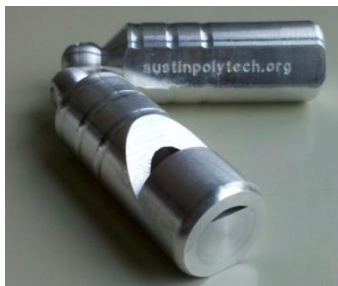
Fully functional aluminum whistles manufactured by APA students.
